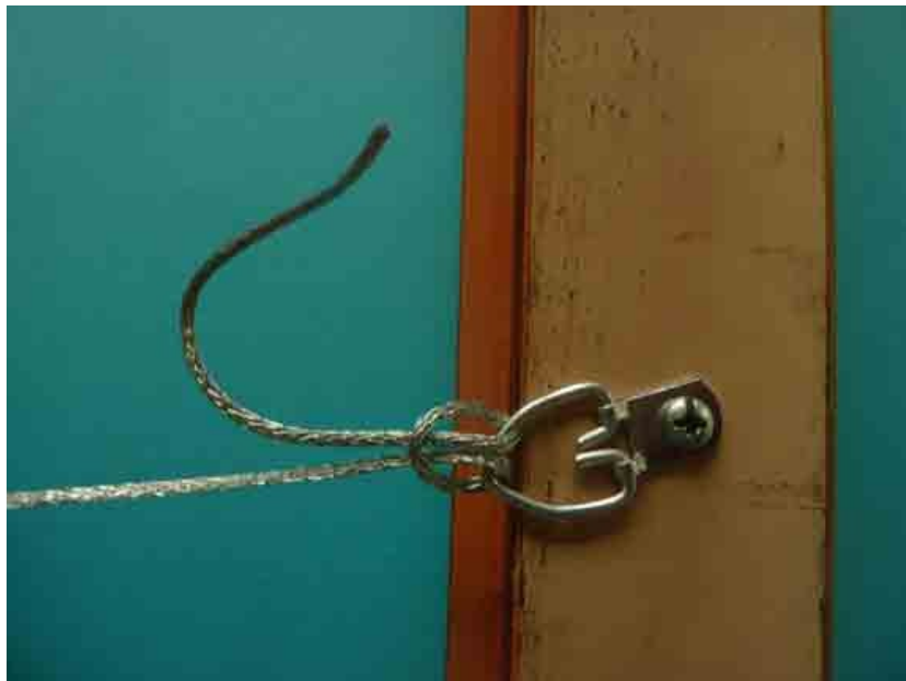
wire tied on to strap hanger
